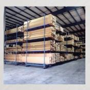
An excellent portable alternative to static pallet racking, stacking racks save valuable space by storing bulk items in individual racks. A safe and economical product, stacking racks are typically constructed using structural materials. Collapsible options make empty stacking racks easy to store in only a fraction of the space used when loaded. Each rack is designed to meet your exact loading requirements.
